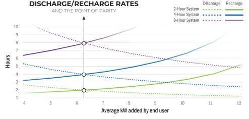
Note: Charge starts at ~30% battery capacity and stops at ~90%. These set points can be adjusted to meet performance requirements.
